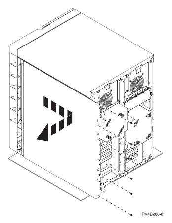
Figure 3. Remove System Unit Side Cover
